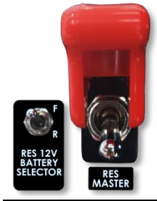
Figure 7-25 RES master switch and 12V battery selector
